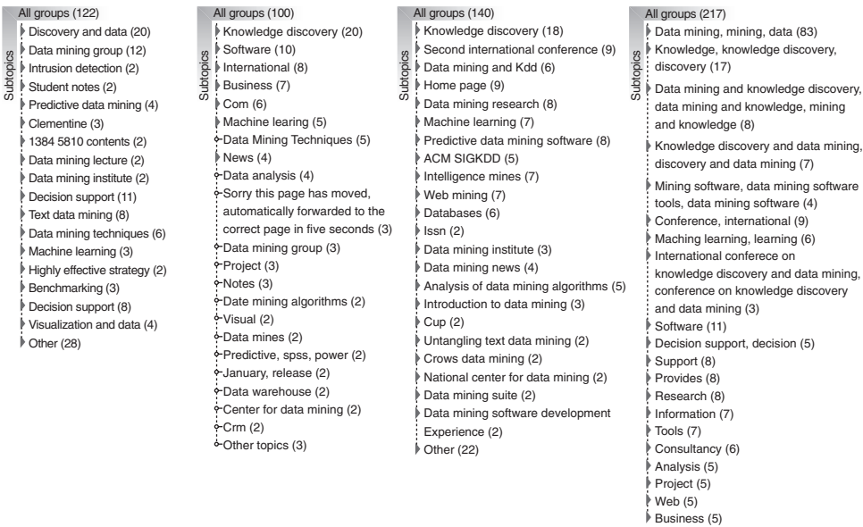
Figure 47.5 Comparison of results for a query ‘data mining’ produced by different algorithm (from left to right): TRC, LINGO, AHC, and STC. All outputs were produced using Carrot 2 visualization component
